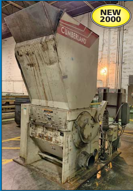
100-HP Cumberland Model X-1000 Plastic Granulator
